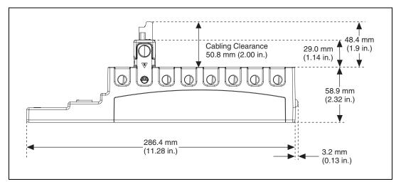
Figure 2. NI 9144 Chassis, Bottom View with Dimensions
